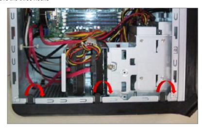
**2.2** Disconnect the cable housing then you can remove front bezel.
